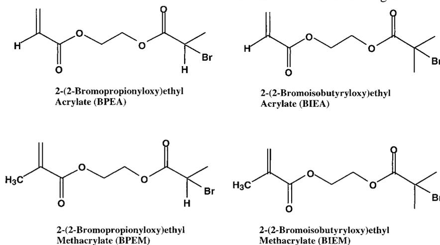
Fig. 1. AB\* (meth)acrylic monomers used for SCVP by ATRP
