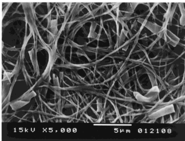
Figure 4. SEM image of fibrous aggregates of GA8 assembled in 5CB after the extraction of 5CB .
