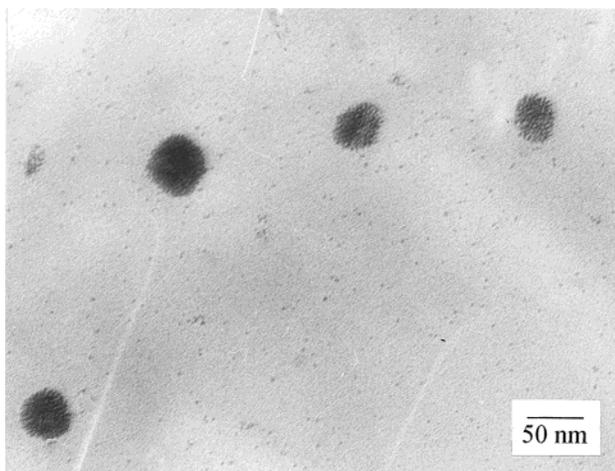
**Figure 3.** TEM micrograph of Pt nanoparticles stabilized in the PS-*b*-PEO/CPC block copolymer micelles in water and obtained via reduction of  $\text{H}_2\text{PtCl}_6 \cdot 6\text{H}_2\text{O}$  ( $1.24 \times 10^{-2}$  mol/L) with  $\text{NaBH}_4$ .
