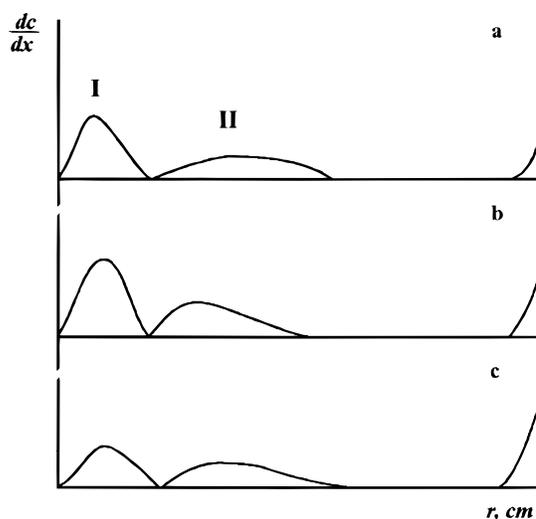
**Figure 1.** Sedimentograms of PS-*b*-PEO in aqueous solutions containing various amounts of CPC:  $0.8 \times 10^{-3}$  (a),  $0.14 \times 10^{-2}$  (b), and  $0.2 \times 10^{-2}$  (c). The PS-*b*-PEO concentration was 0.5 g/L. Here and in Figure 2, rotation rate was 50 000 rpm and time was 30 min (from the beginning of rotation). Characteristic sedimentation coefficients ( $S_0$ ) for the main peaks I and II (for Figures 1 and 2) are presented in Table 4.
