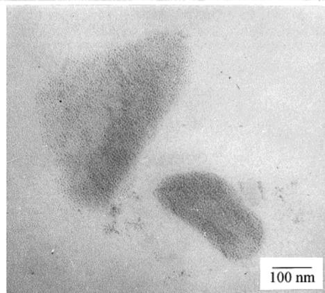
**Figure 4.** TEM micrographs of Pt nanoparticles stabilized in the PS-*b*-PEO/CPC block copolymer micelles in water and obtained via reduction of  $\text{H}_2\text{PtCl}_6 \cdot 6\text{H}_2\text{O}$  ( $3.36 \times 10^{-3}$  mol/L) with molecular hydrogen.
